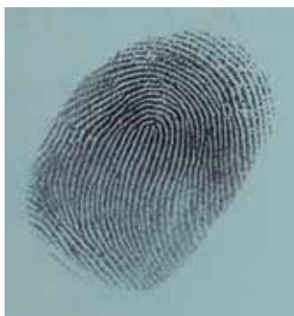
Fig. 3 A Fingerprint developed on a glass article after 36 hours of immersion in water
