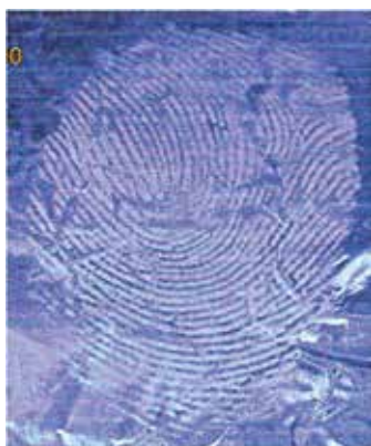
Fig. 4 A Fingerprint developed on aluminium foil after 7 hours of immersion in water
